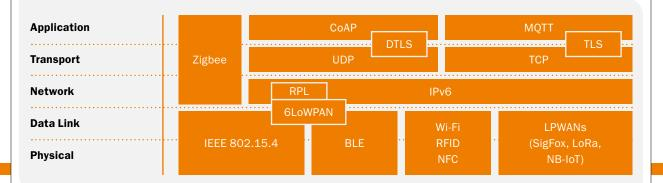
Figure 24: IoT Network Protocol Stack\* (\*integration of LPWANs with IPv6 is under way at IETF<sup>243</sup>)
