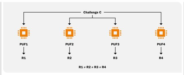
Figure 17: Physical Unclonable Function (PUF)
